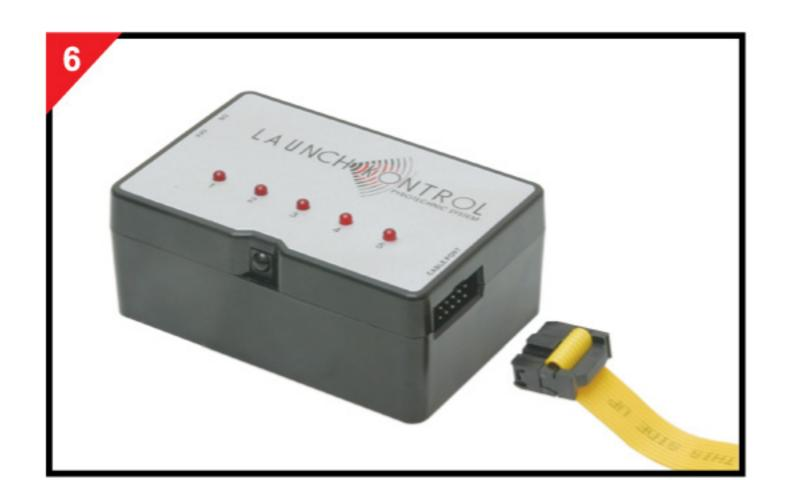
To activate transmitter press and hold the SET UP BUTTON until the red MODE LIGHT illuminates. The transmitter has 4 firing channels A B C and D.
